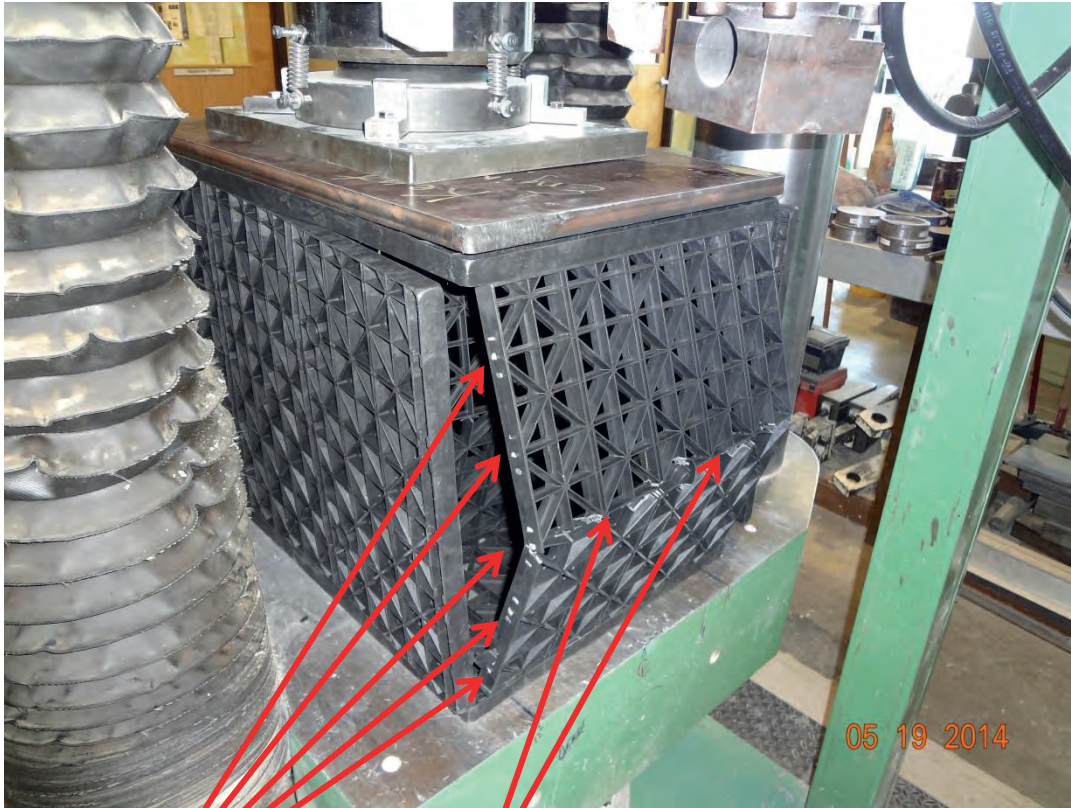
Figure 9: First test block failure from the back side
