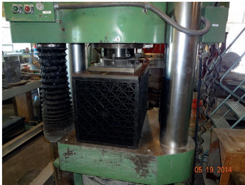
Figure 2: Test machine with steel plate on the test block.
